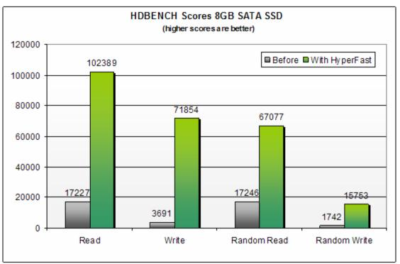
Figure 3: Benchmark scores on 8GB SATA SSD with HDBench™ software.
