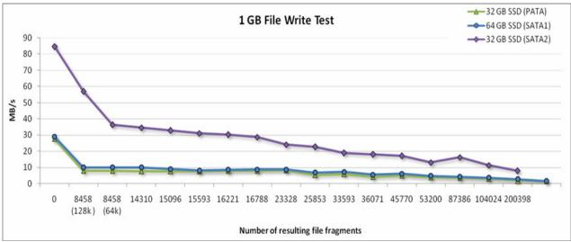
Figure 2: Write I/O throughput degredation due to fragmented free space.
