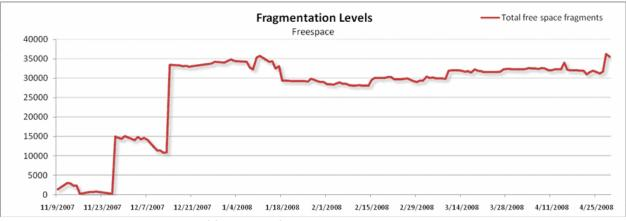
Figure 1: Accumulation of free space fragmentation through normal system use.
