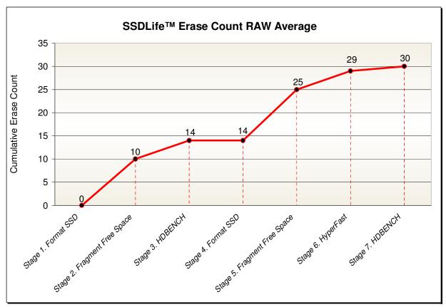
Figure 7: Cumulative Erase activity on 8GB PATA SSD as measured by SSDlife software.
